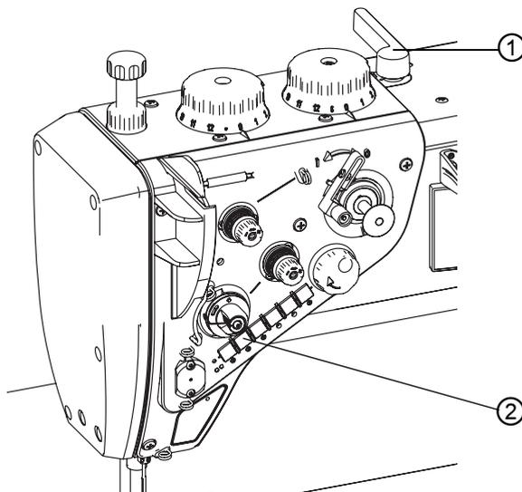
(1) - Hand lever for lifting presser foot
