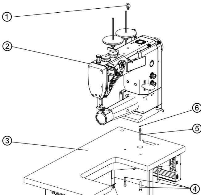
(1) - Suspension screw with eyelet
