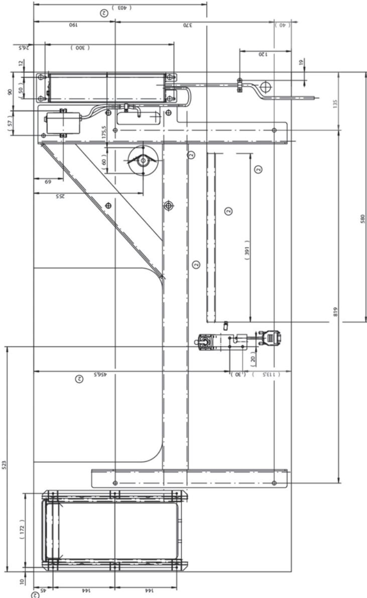
Fig. 59: Components on underside of the folding table plate
